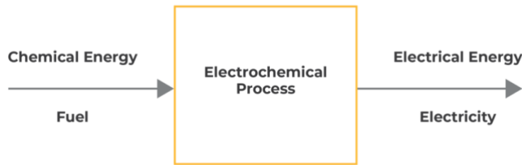
Figure 1: Energy Schematic of a Fuel Cell
